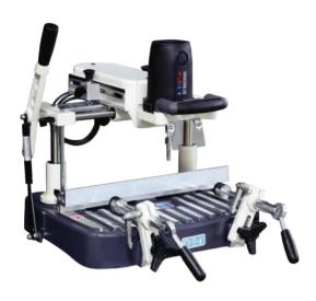
Used for cutting appropriate slots on aluminum and plastic profiles for mounting locks, grips, hinges, latches and opening channels.
