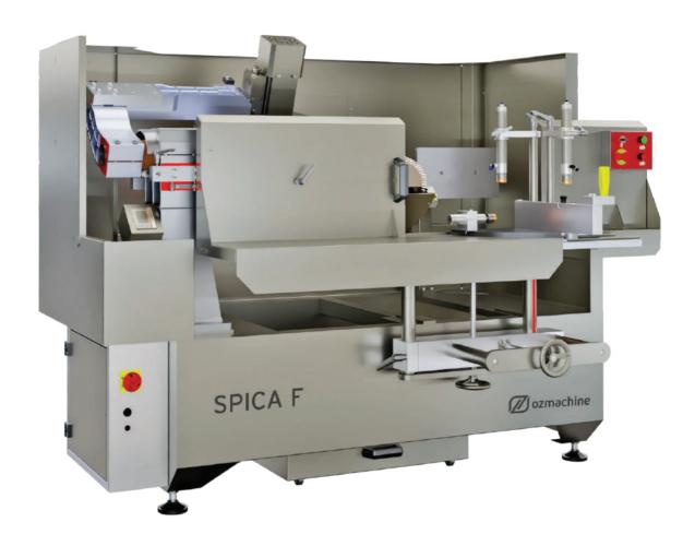
SPICA F saw Notching Machine is designed and constructed for variable notching possibilities on the sash, frame, mullion and transom profile combinations for curtainwalls, winter gardens, skylights and special design processing with the special angles at the profile and surface. A work unit that moves on a profile fixed with automatic horizontal and vertical clamps, which is controlled manually via a linear guide slide, performs cutting operations using two fixed saws.
