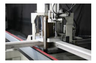
Through its electronic thermostat heat adjustment between 0°C - 350°C, welding time adjustment and digital controlled heat, quadruple welding unit provides scattering homogenised to plaque of heat.
