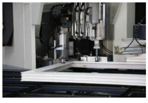
11 pieces of profile cleaning blade and two independed cleaning unit, cleaning bottom, top, interior and external surfaces of the profile.
