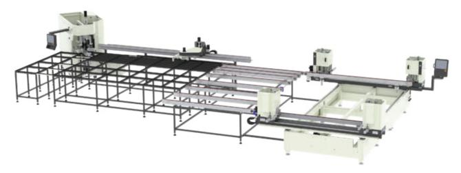
**SIRIUS** which is the line of Automatic PVC welding and edge cleaning has been developed for cleaning processes occuring in profile after welding and welding at the same time of four edges of plastic profiles. With automatic frame unloading unit, fast transfer to cleaning unit of profile with robot system and with the system of automatic profile rotating, **SIRIUS** gains time substantially while decreasing workload on user in welding and cleaning processes.
