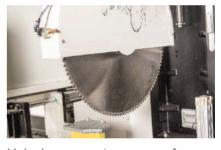
Unlock a vast array of cutting possibilities with the unit's 550mm diameter saw blade, capable of tackling any angle between 30° and 150°. This expansive cutting range empowers users to maximize their creative and production potential.
